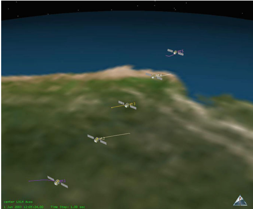
Fig. 5.15 Satellite motion under decentralized formation control to maintain in-plane formation
