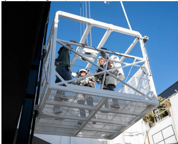
Figure 4. In 2023, NASA astronauts Nicole Mann and Doug Wheelock tested a subscale mock-up of the elevator that will take crew from the airlock deck to the lunar surface in the Starship HLS during Artemis III and Artemis IV. (Image credit: SpaceX)
